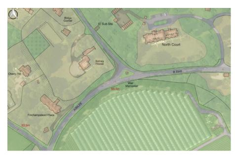
The junction is physically too narrow for two vehicles to pass on the northeast side of the Memorial when travelling from the California Crossroads to The Ridges. Due to the topography and construction, the road has a blind bend where Jubilee Road and Rectory Hill meet to the west of the Memorial.
